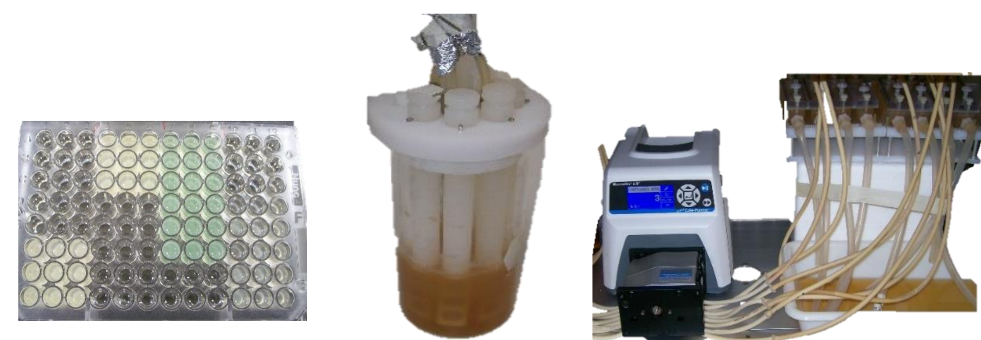
Figure 1. Photographs of an MBEC device (left), CDC reactor (centre) and Drip Flow reactor (right).
